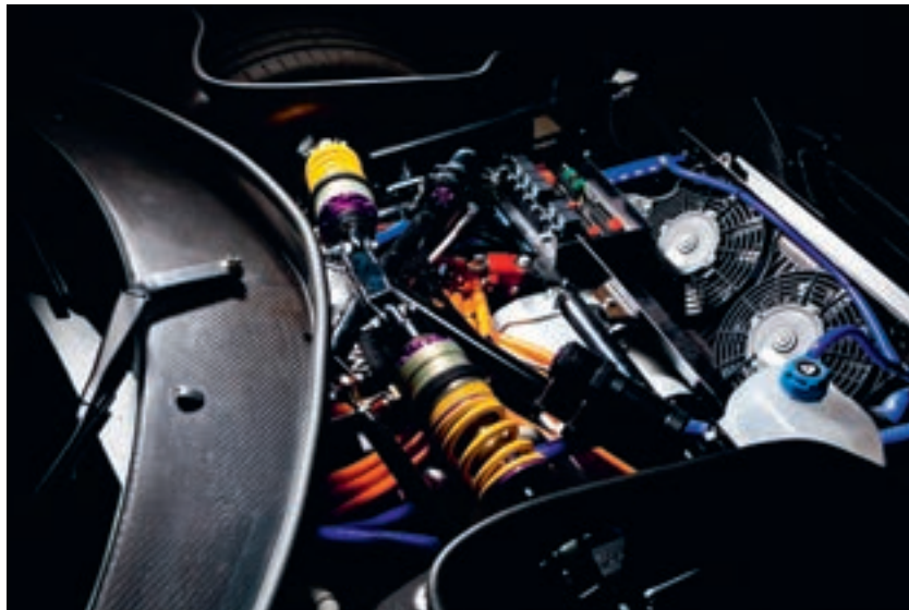
The Concept_One is built around a unique powertrain and battery pack that the Rimac team developed from scratch.
